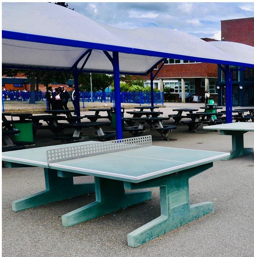
Image 2: pigmented green tables are steel reinforced precast concrete, with aluminium hole punched net. No annual maintenance. 25 year warranty.
