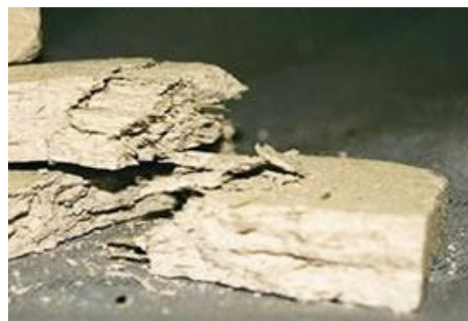
Pieces of Asbestos Insulating Board (AIB)
